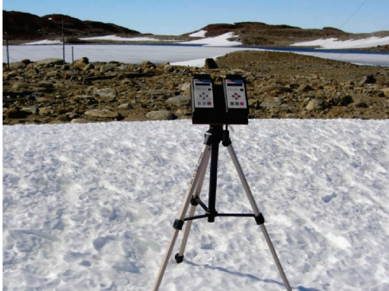
Fig.1: Photograph of Microtops II (Sun photometer and Ozonometer) operating at Maitri
