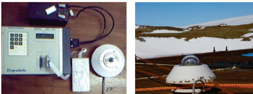
Fig. 2: Photograph of the global short-wave radiometer with data acquisition system. Location of the sensor in the Antarctic environment can also be seen in the figure.
