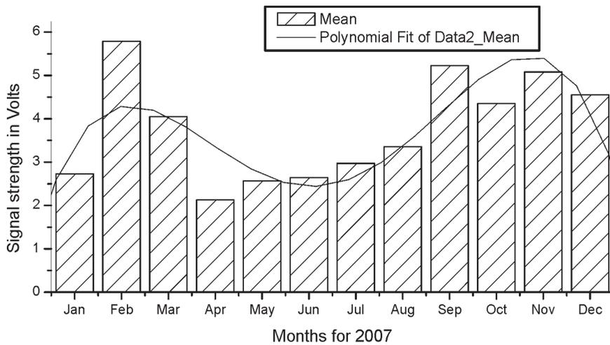
*Fig. 5: Monthly mean value of Riometer signal strength for the year 2007*
