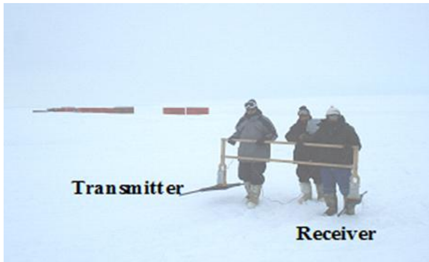
Fig. 2: Use of 50 MHz unshielded GPR antenna for ice depth estimation at Shelf ice
