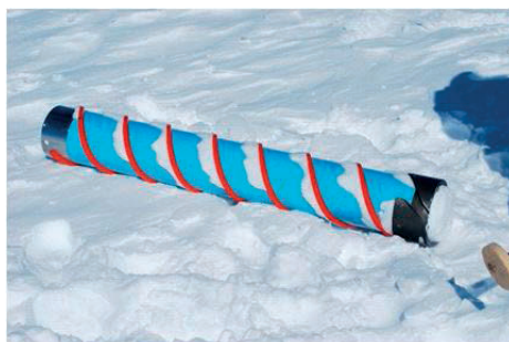
Fig.2: Snow coring with KOVACS Mark IV Coring system.
