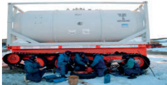
“Logistic personnel trying to find the defect in the Wheel Hub of TIS Axle Trailers”
