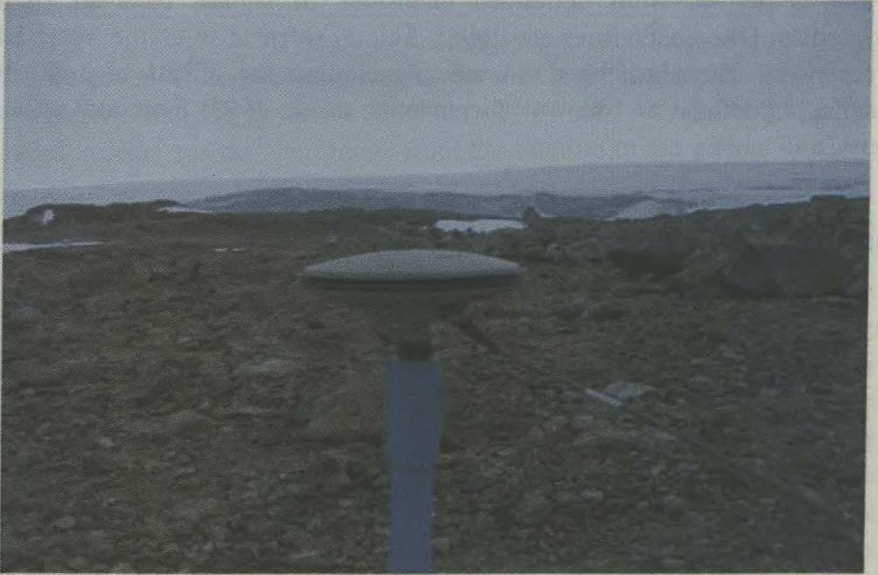
Fig. 1: GISTM (GSV4004A) antenna installed at MAITRI, during 25 th Indian Antarctic Expedition
