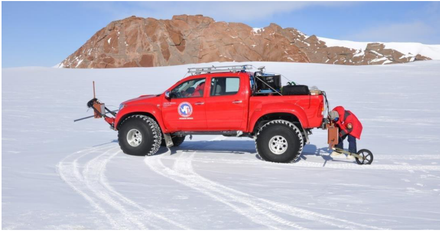
Fig. 3. GPR survey using the snow vehicle (Arctic Truck) with fitted Transmitter (Tx) and a Receiver (Rx) inside a wooden box at the rear side and front side respectively. Tx is attached with a survey wheel towards the rear side of the vehicle.
