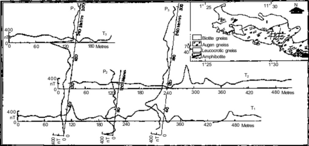
Fig 3 Profiles showing magnetic response over augen gneiss - Schimacher Hill region. The geological details are from Sengupta 1986 (this volume).
