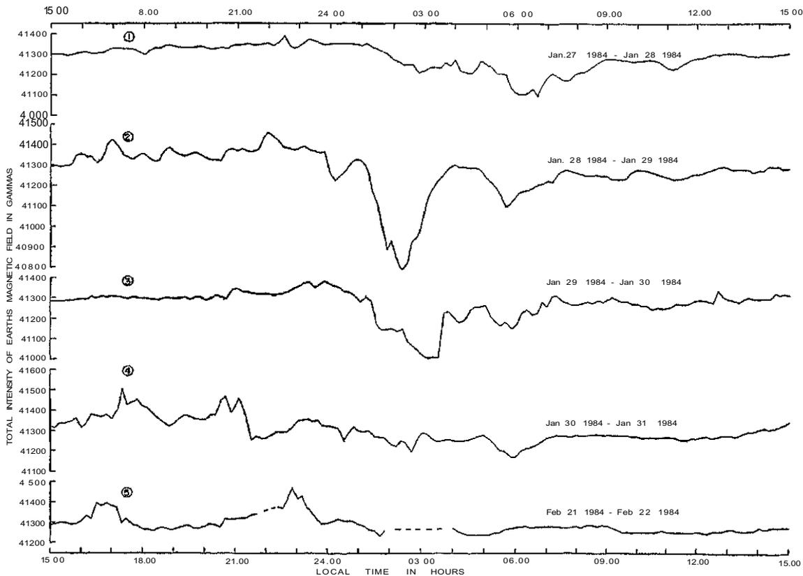
Fig 1. The earth's intensity magnetic field measurements at the Schirmacher Hill and at the Base Station
