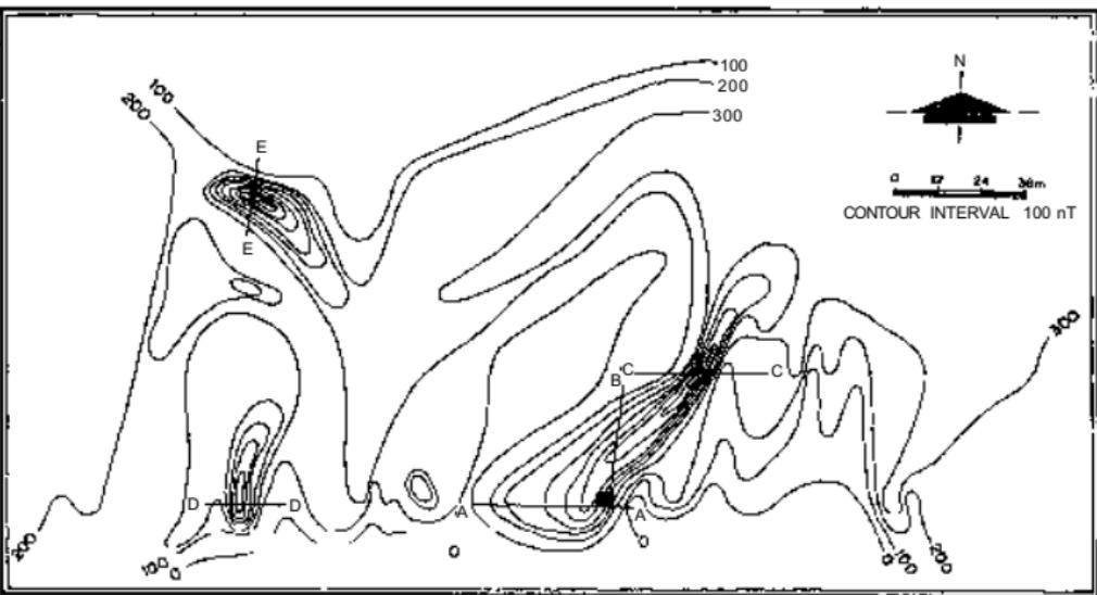
Fig 4 Magnetic intensity contour map to demonstrate the influence of shallow intrusives on magnetic measurements over augen gneiss Schimacher Hill. Profiles AA BB CC DD and EE are considered for quantitative interpretation.
