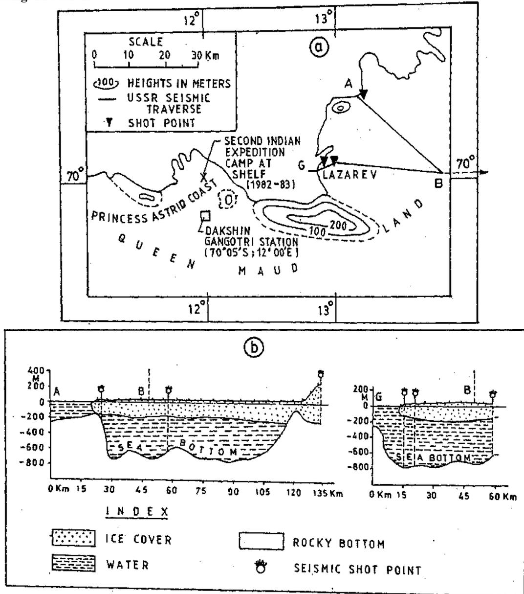
Fig. 6. (a) Depth of the bedrock near the Lazarev Coast, Queen Maud Land, (b) seismic sections (After Atlas Antartiki, Vol. 1, 1966).
