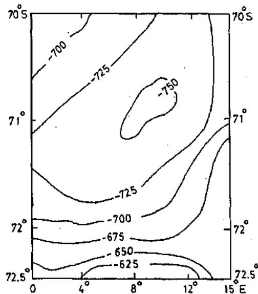
Fig. 5. Extracted bedrock elevation contours in Dronning Maud Land region.
