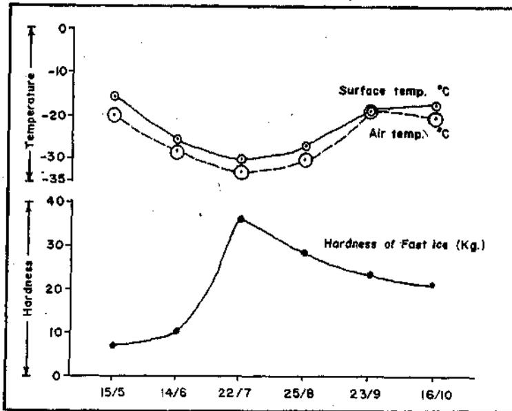
Fig. 33. Variation in ramsonde hardness of fast ice from 15.5.86 to 16.10.86
