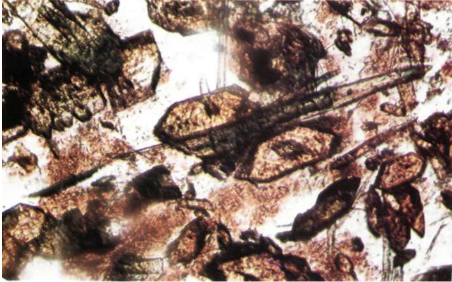
Fig. 5a. Photomicrograph showing typical pandomorphic texture depicted by zoned clinopyroxenes set in a groundmass rich in feldspars (O.L., 50x).
