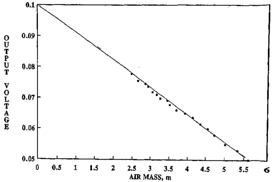
Fig. 12c. Langley plot for 675 nm.
