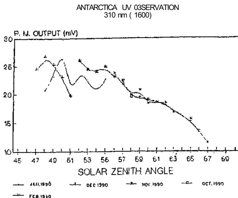
Fig. 6. Variation of solar intensity at 310 nm (in the form of photomultiplier tube output) with solar zenith angle for the different periods of 1990.
