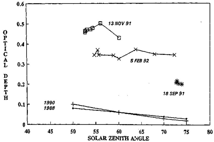
Fig. 10b. Variation of optical depth with solar zenith angle for 500 nm.
