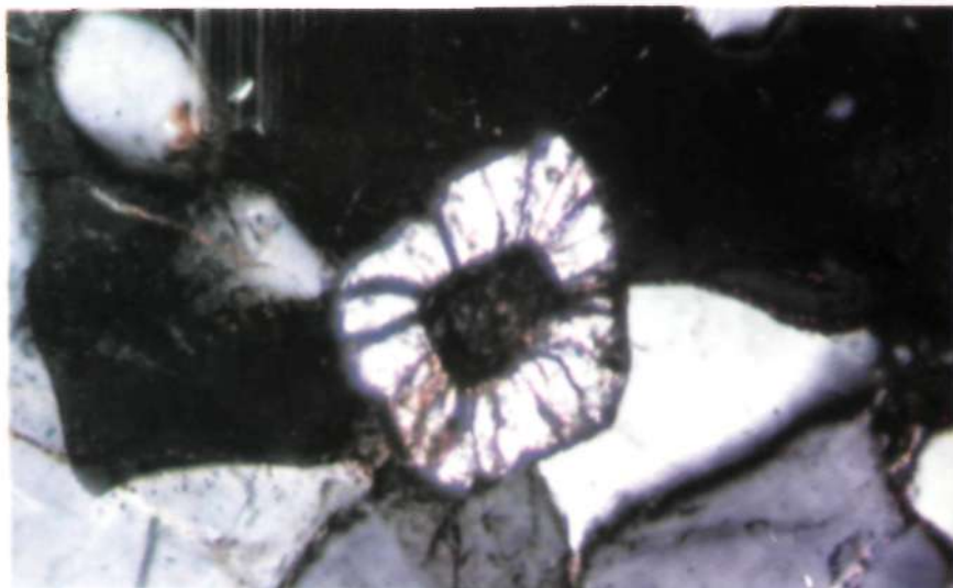
Figs.6 & 6A. Photomicrographs in plane polarised light and under cross nicols (20X) showing euhedral allnite in foliated granite.
