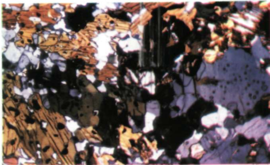
Figs. 5 & 5A. Photomicrographs in plane polarised light and under cross nicols (4x) showing presence of orthopyroxene and clinopyroxene along with other mafics and opaques clustered together in foliated granite.
