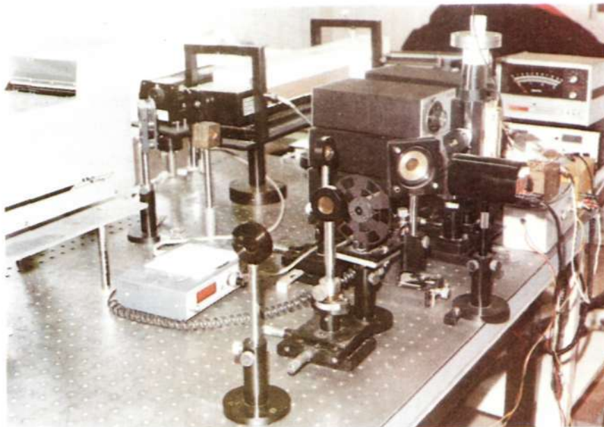
2. Laser heterodyne system (NPL) installed in Maitri
