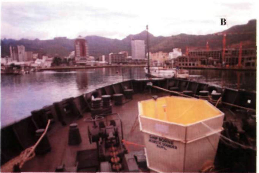
Fig. 2: (A) Shipborne acoustic sounder being installed onboard the ship M. V. Thuleland. It was built around a 6 feet parabolic dish seen in the photograph. (B) The shield installed onboard the ship M. S. Brinknes in the bow region. The 4 feet parabolic dish is inside the shield placed on a gyrostabilised platform
