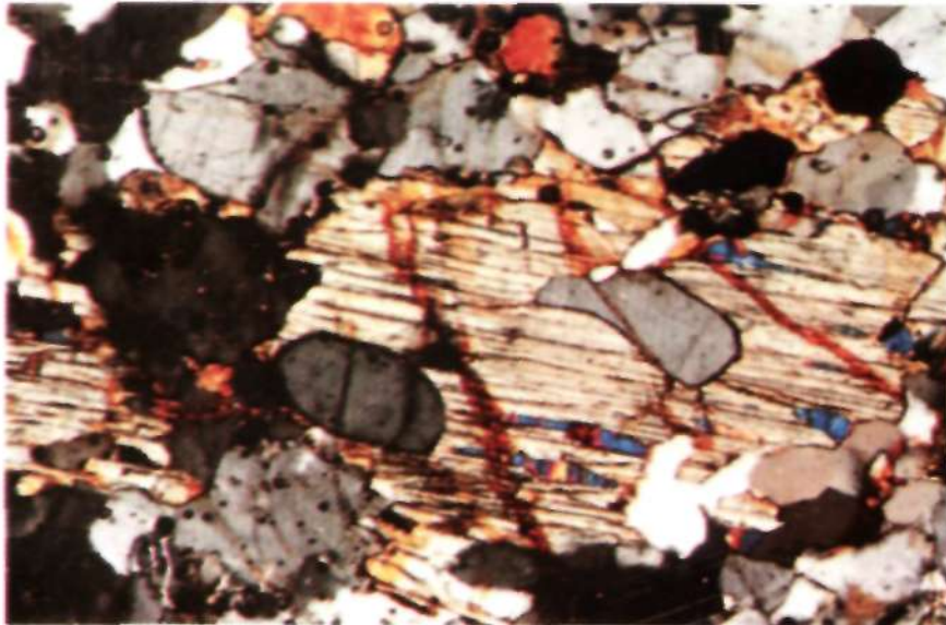
Fig. 7: Orthopyroxene showing exsolution lamellae of cpx along cleavage plane in gneissic charnockite with included apatite (x 40)
