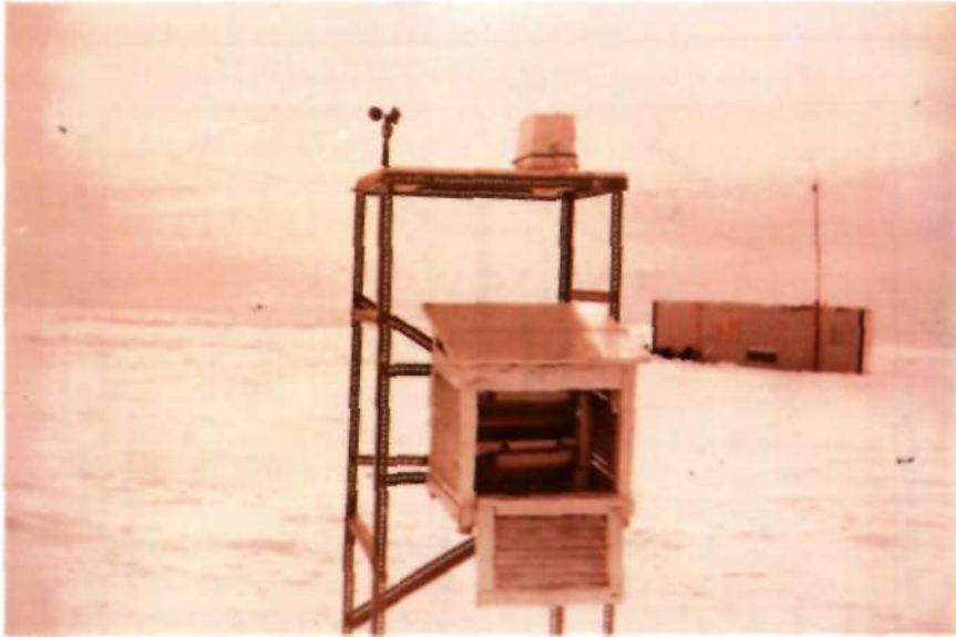
Photo 2(a) : 2.5 meter tower containing Pyranograph. Anemometer and Stevenson Screen at D.G.
