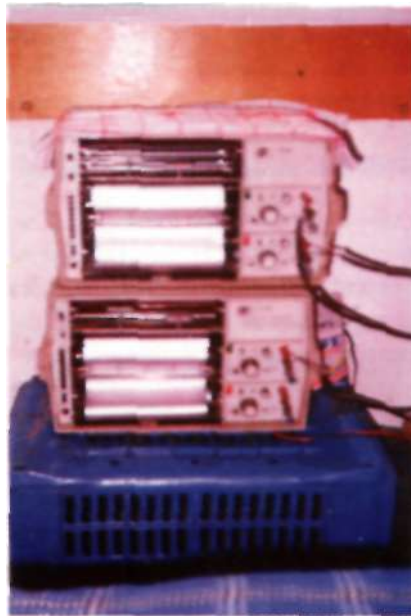
Photo 1(b): Electropoly recorders (EPR) with silver coated electrosensitive charts used for continuous recording of integrated albedo and net radiation
