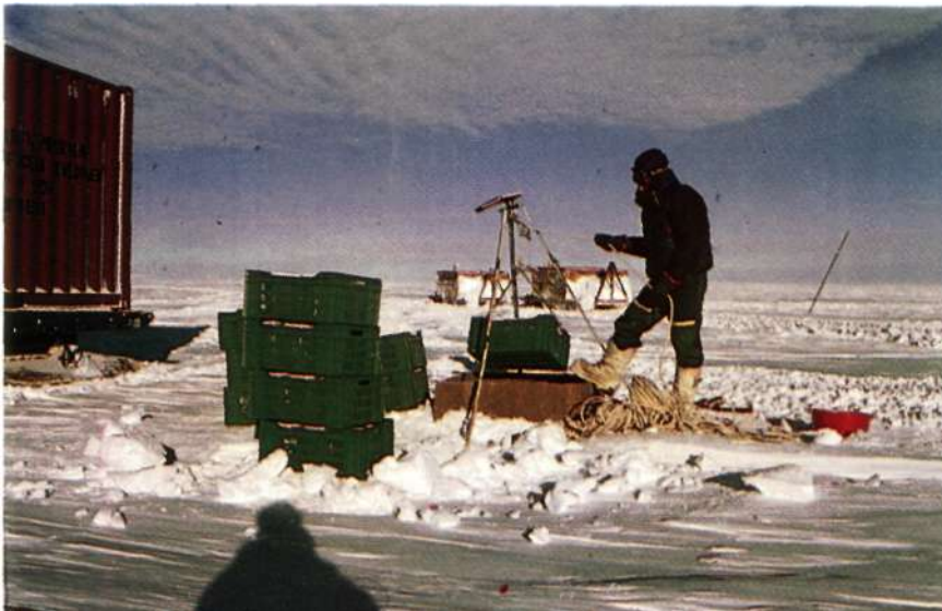
Fig. 11 : Core being lowered in Dakshin Gangotri hanger building below the surface
