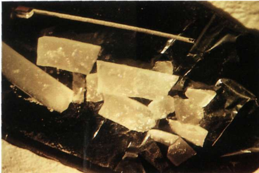
Fig.3 : Core from bottom of first borehole that exploded spontaneously
