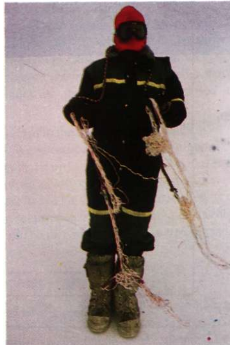
Fig. 14 : Even the 3000 kg load-capacity mountaineering ropes are smashed
