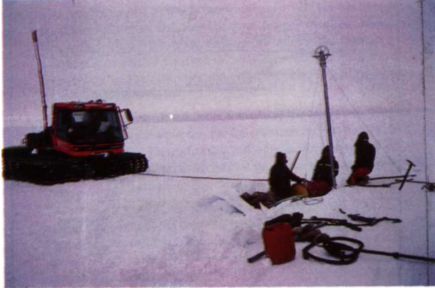
Fig. 13 : Attempt to retrieve the stuck drill barrel by pulling with a vehicle
