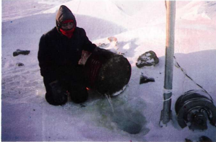
Fig. 1 : The borehole being filled up with water, after installing 14 thermistors
