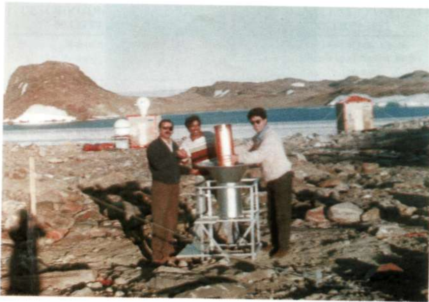
Plate-3 Snowgauge installed during Summer of 1998
