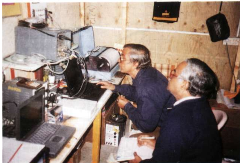
Fig 2. Ashtech Z-XII GPS Receiver and on site computer installed inside the Tirumala Hut.
