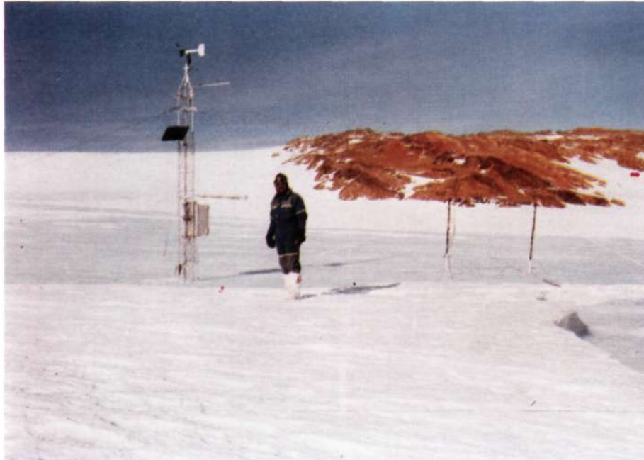
Automatic weather station (AWS) set up on Polar Ice at Sankalp Point
