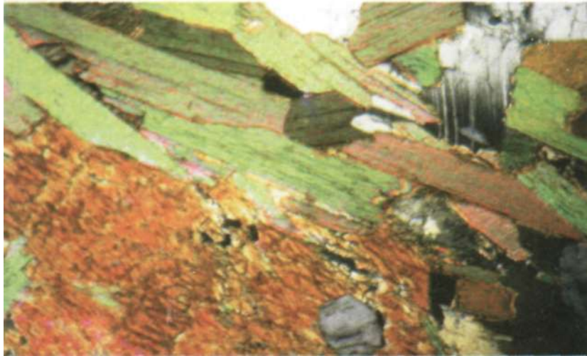
Fig. 5: Biotite and hornblende grains defining foliation in the hbl-bio-bearing orthogneiss from the nunatak Sonstebymuten (crossed nicols; 10x).
