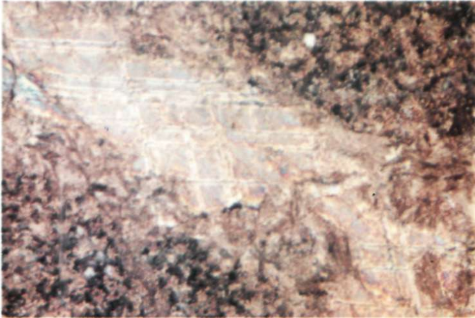
Fig.4. Photomicrograph of limestone from Moltke Nunataks, Weddell Sea, coarse calcite vein cuts across the slide, x 20.
