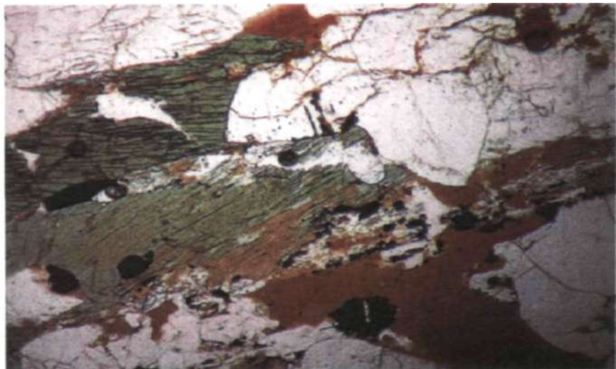
Fig. 3 Secondary biotite forming at the expense of hornblende with concomitant exsolution of opaques in the hbl-bio-bearing orthogneiss from Baalsrudfjellet (plane polarized light ; 10x)
