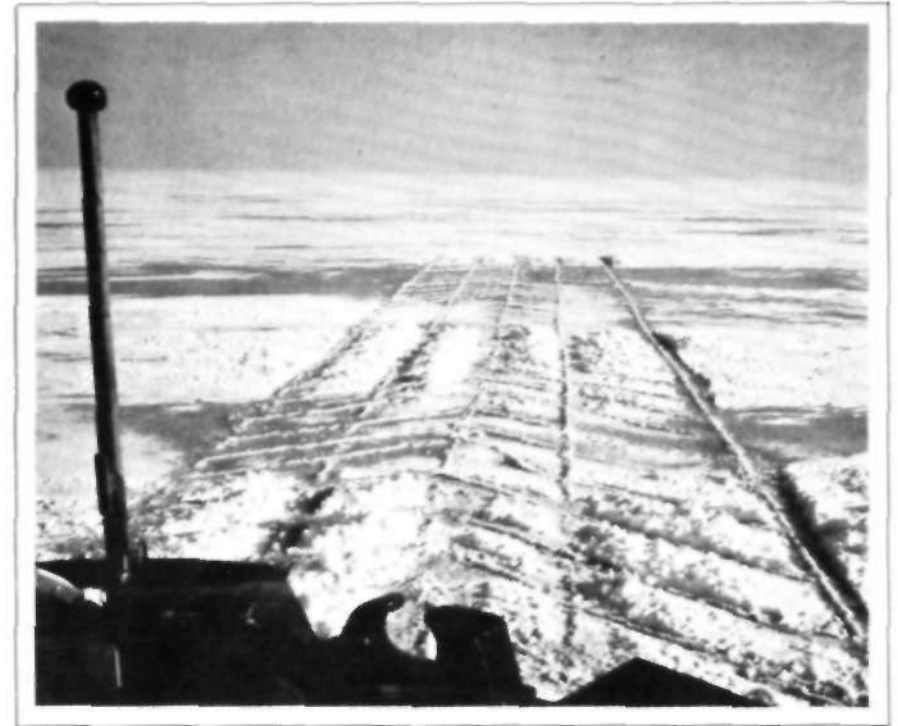
A FULL-SCALE TEST IN A PRE-SAWN ICE FIELD UNDERTAKEN TO STUDY THE COMPONENTS OF ICE RECITANCE.
