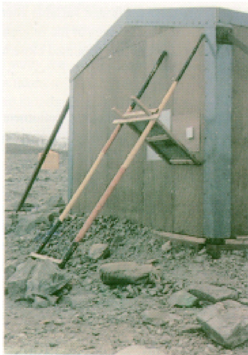
Fig 2 : Position of metallic reflector kept at 45° to the ground outside the hut, aligned to the radiometer antenna.
