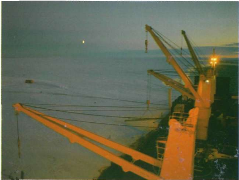
Fig. 3: Ship on shelf-notice the crane size reaching just the shelf edge.
