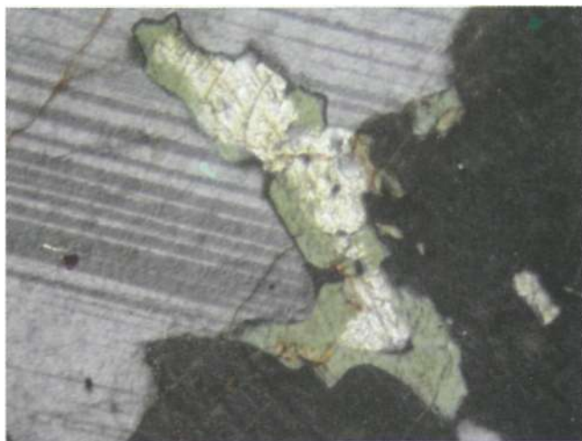
Fig. 7: Retrogression of clinopyroxene to hornblende
