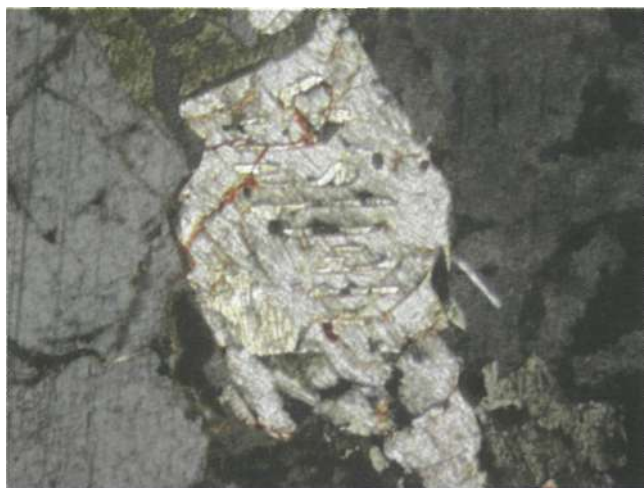
Fig. 6: Inverted pigeonite in charnockite sample No. 9/XXI
