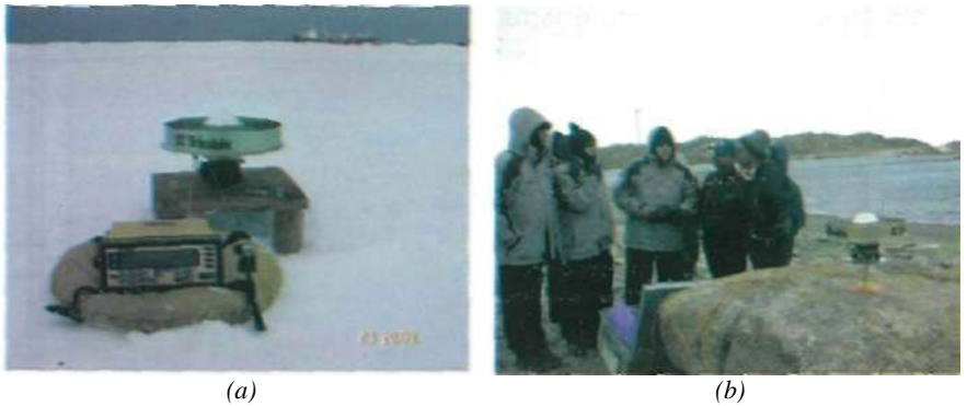
Fig. 4: Photos show (a) GPS antenna mounted on wooden platform fixed on the glacier and (b) GPS base station set up on exposed bedrock near the Maitri station
