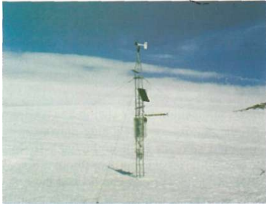
Fig. 5: AWS installed near Sankalp Point
