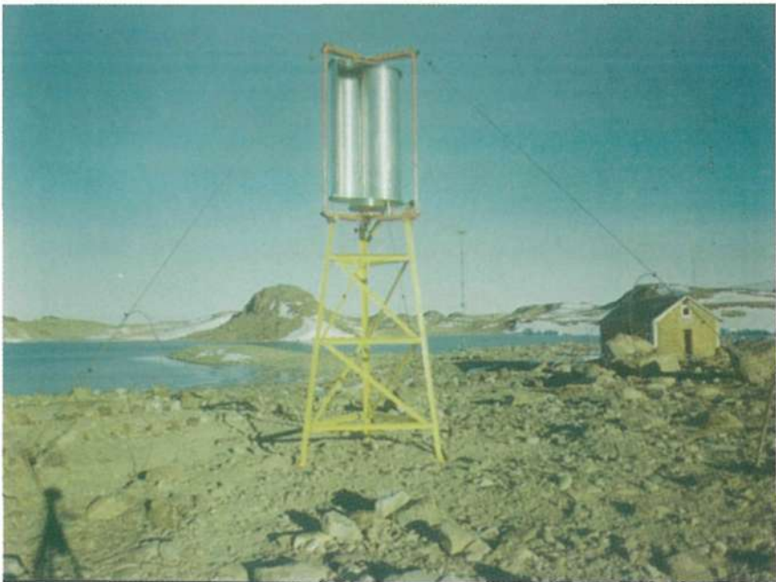
Fig. 3: Savonius Wind battery charger near Arravalli hut
