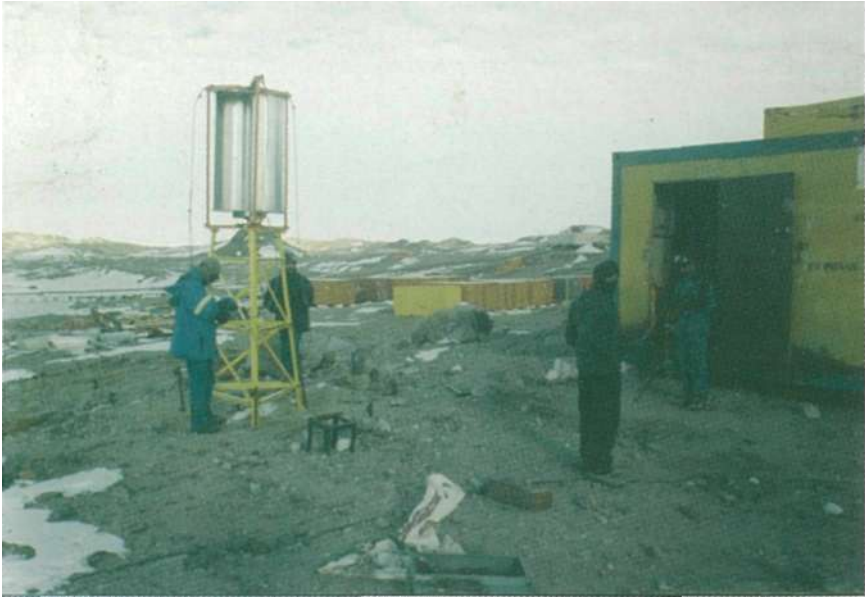
Fig. 2: Savonius Wind battery charger near station work shop
