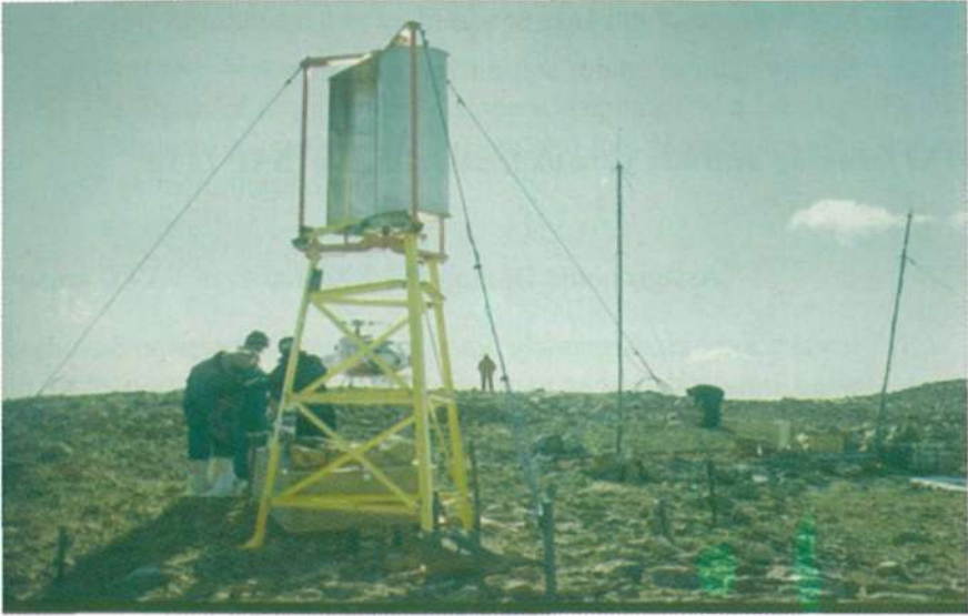
Fig. 1: Savonius Wind battery charger at Vattiah peak
