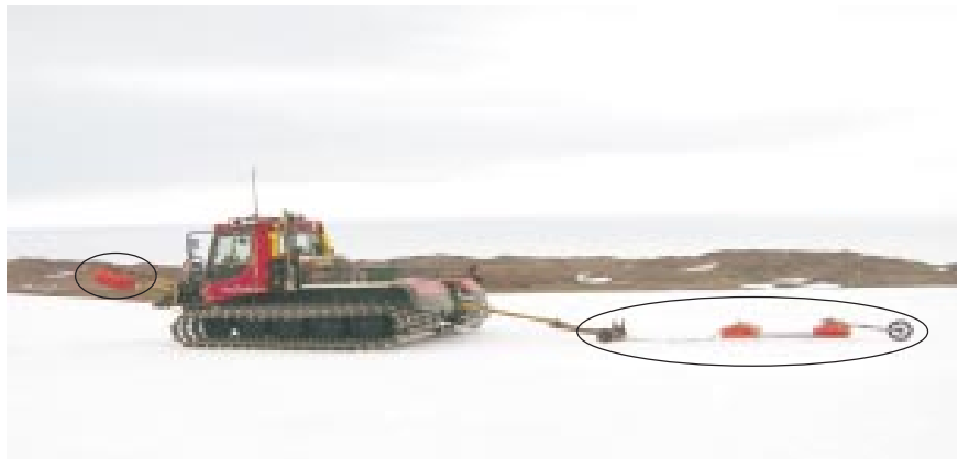
Fig. 34 : Brackets mounted on Pisten Bulley for installing GPR devices
