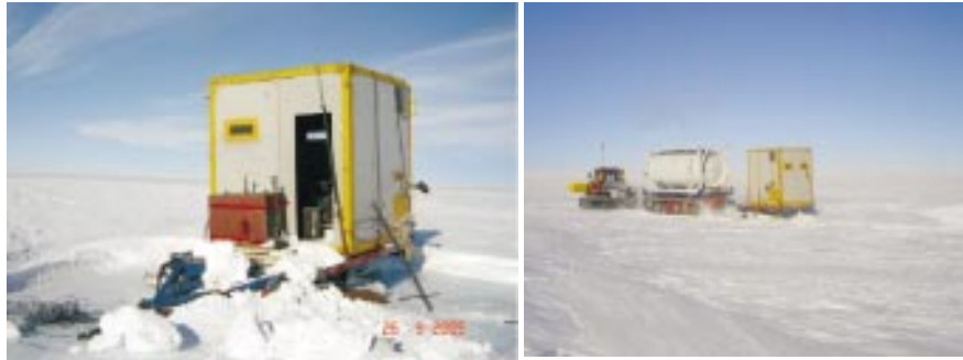
Fig. 11 : Fabricated generator module and its double towing along with tanker load
