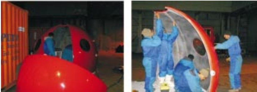
Fig. 13 : Assembly of apple hut in the ship's hold
