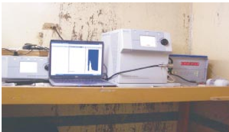
Fig. 1 : The Aerodynamic Particle Sizer (APS) and Scanning Mobility Particle Sizer (SMPS) systems installed inside the Kamet hut at Maitri
