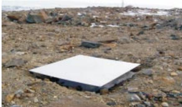
*Fig. 2 : Air-earth current plate antenna installed at Maitri*
