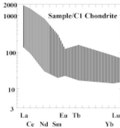
Fig. 10a : Chondrite normalized REE spidergram for granite (normalizing value after Nakamura 1977)
