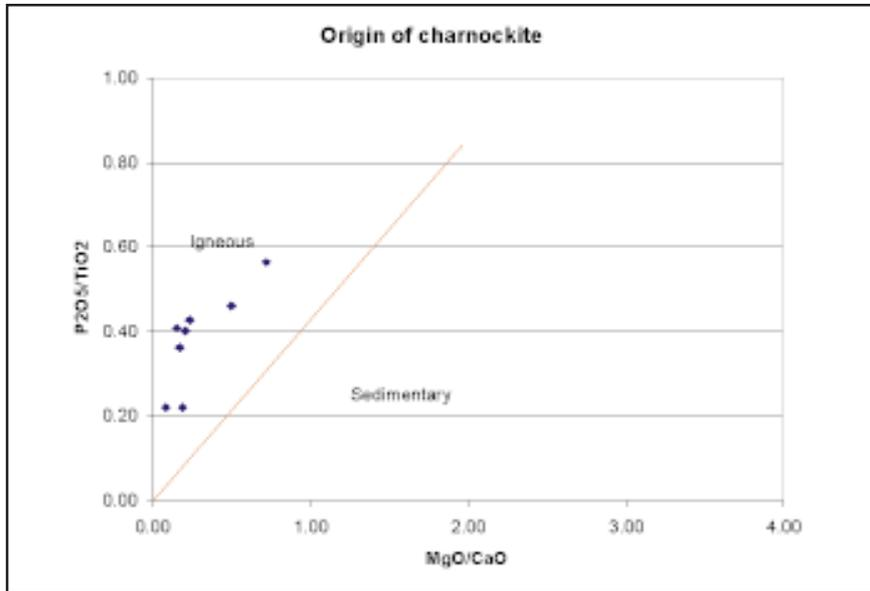
Fig. 11 : Plot between  $P2O5/TiO2$  vs  $MgO/CaO$  (wt%) (Harker, 1909) for origin of charnockite
