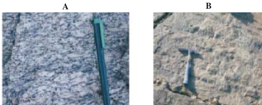
Fig. 4 : Hand specimen of gneiss rock shows the coarse grain and lineation alignment of feldspar, quartz, biotite and garnet
