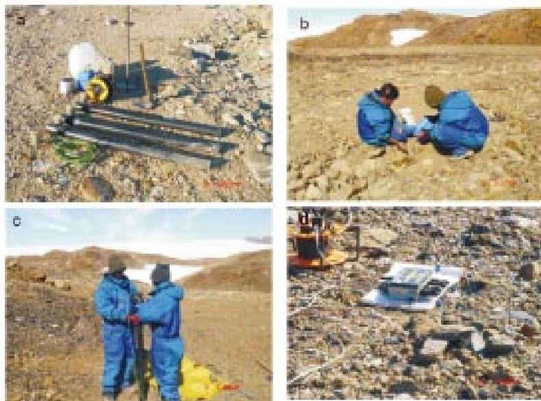
Fig. 14 : (a) Induction coil, porous pot assembly (b) Fixing of Cd C12 Porous Pot at MT site (c) Leveling and positioning induction coil (d) Signal Detection Box during data acquisition
