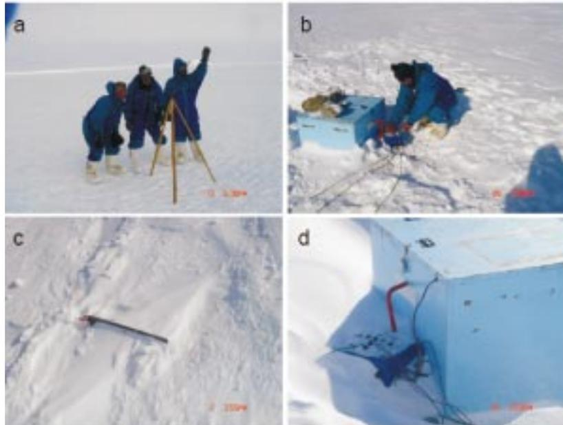
Fig. 13 : (a) Fixing layout on ice station (b) Inspection of equipment during the recording (c) Titanic sheet as electrode and (d) ADU-06 covered with ice after 6 days
