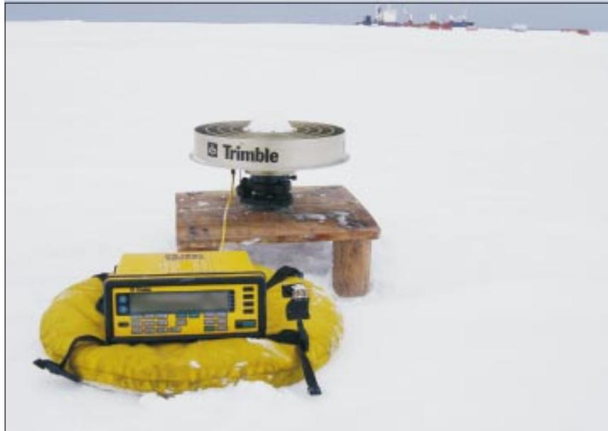
*Fig. 3 : GPS antenna mounted on wooden platform which is embedded in the glacier at DG GPS location. The ship used in the expedition is moored on the shelf is seen at the background*
