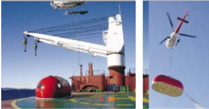
Fig. 1 : Assembled Melon Hut on the heli-deck and airlifting by the helicopter
